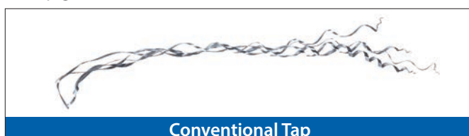
■ Chip generated in 40m/min
