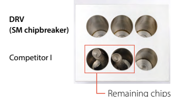
Comparison of remaining chips (In-house evaluation)
